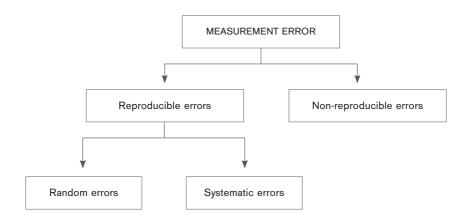
There are many potential causes of measurement errors, which are divided into reproducible and non-reproducible errors. Technically, the latter should never arise during analysis, but in fact they are time and again the cause of false assessments of the situation. Typical examples include the use of measurement equipment that is not suitable for the application, or measurements taken in the wrong place. Reproducible errors are divided into random errors and systematic errors.
