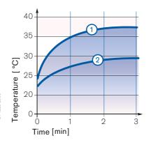
Cooling effect of the hot air probe gas temperature: 650 °C ambient temperature: 20 °C In 3 minutes 1 L of gas was drawn and the temperature in the tube rose according to the above curves (1) with one hot air probe
