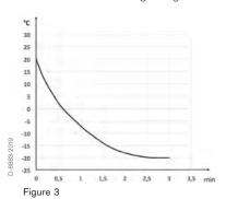
Figure 3 shows a cooling curve recorded at an ambient temperature of -20 °C. The temperature was measured at the beginning of the tube filling. After 3 minutes a liter of cold air was drawn through the tube constantly. The detector tube (which was previously at a temperature of +20 °C) was exposed directly to the cold ambient air. After a minute the temperature dropped to below 0 °C.
