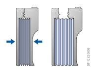
Quick test to evaluate the suction capacity of the bellows pump
