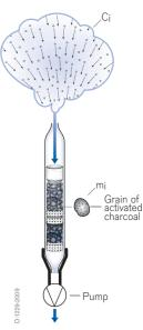
Measurement principle of active sampling with Dräger activated charcoal tubes
