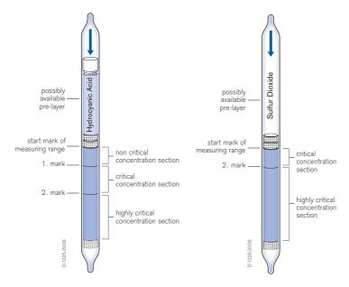
Simultaneous Test-Set II there is a special evaluation of the Dräger-Tubes for chlorine, phosgene and sulfur dioxide. On these tubes, the second mark is missing.
