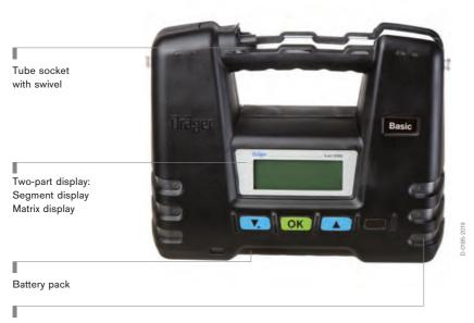
Flashing LEDs: green = end of measurement red = error
