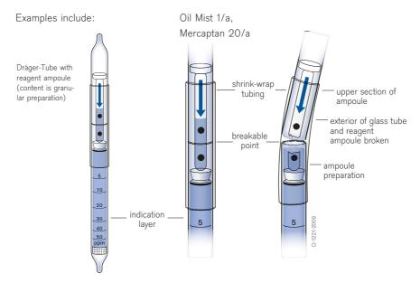
Dräger-Tube with built-in reagent ampoule
