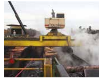
Operators cannot see through the steam cloud caused by condensation in cooler air temperatures.
