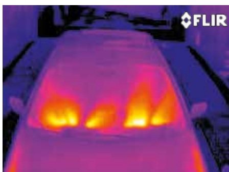
Inspection of car windscreen defrosting.
