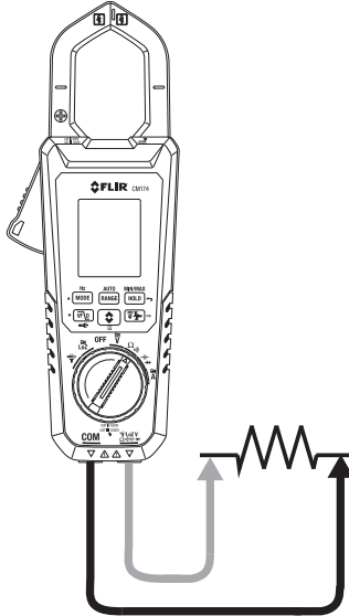
Figure 5.5 Resistance and Continuity Measurements
