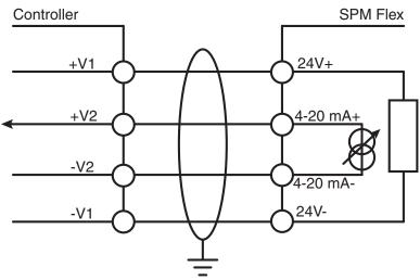
Figure 12. 4-20 mA isolated wiring diagram
