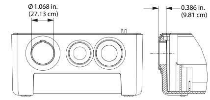
Figure 8. Ethernet opening dimensions
