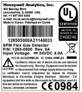
Figure 30. The detector's nameplate
