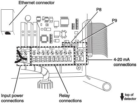
Figure 9. SPM Flex connections
