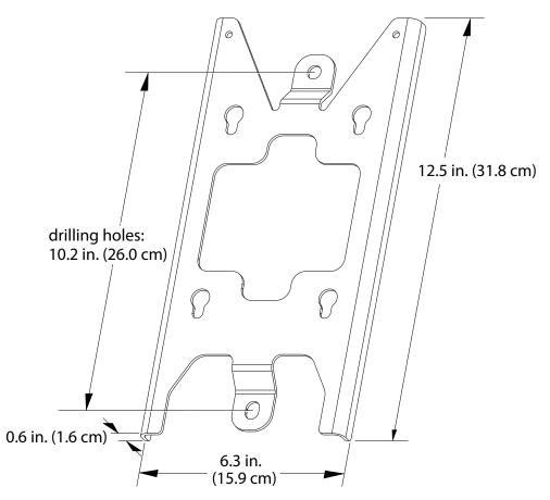
Figure 20. Standard mounting bracket
