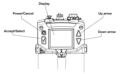
Figure 5. SPM Flex controls
