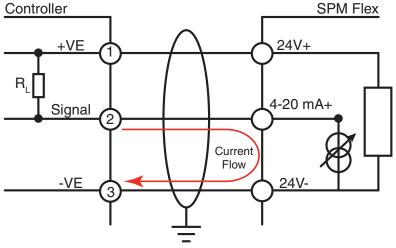
Figure 10. 4-20 mA sink wiring diagram
