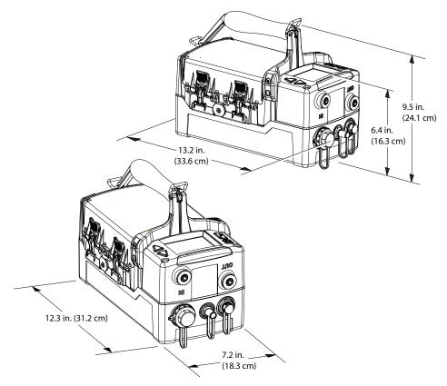
Figure 19. Dimensions of the SPM Flex Gas Detector
