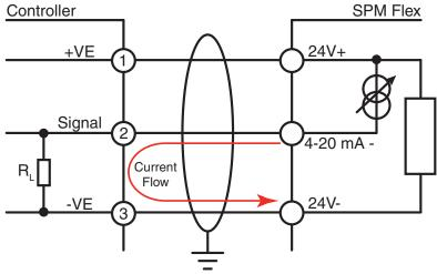
Figure 11. 4-20 mA source wiring diagram
