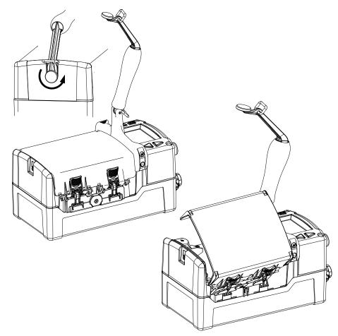
Figure 2. Opening the detector cover
