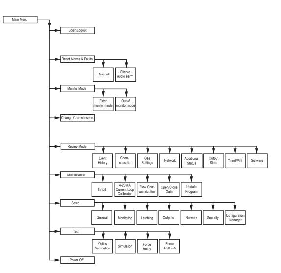
The SPM Flex detector's menus are easily navigated. As an example, this is how a user could review the detector's gas settings when starting from the In Monitor screen:
