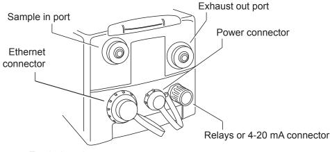
Figure 1. Terminals and ports
