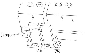
Figure 15. 4-20 mA isolated configuration (the default)
