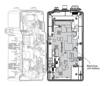
Figure 28. The real-time coin battery
