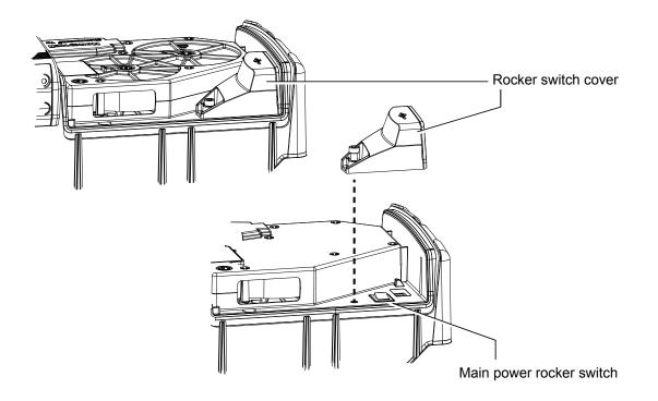
Figure 3. SPM Flex main power rocker switch
