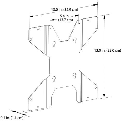
Figure 21. Backward-compatible mounting bracket
