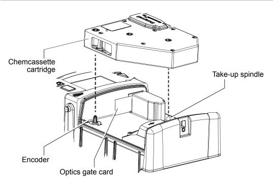
Figure 7. The optics gate card and Chemcassette cartridge
