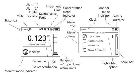
Figure 6. Elements of typical SPM Flex detector displays
