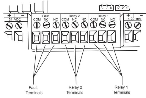
Figure 16. Relay configuration
