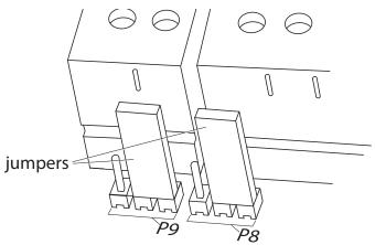
Figure 14. 4-20 mA source configuration
