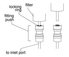
Figure 26. Removing a filter from a push fitting
