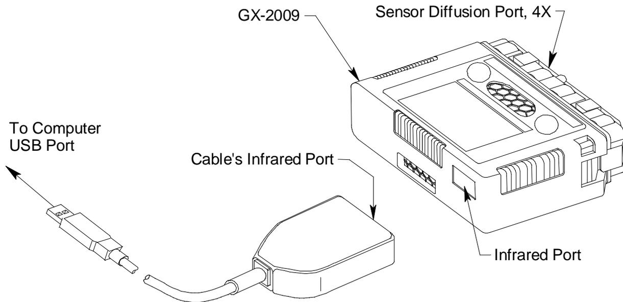
**Figure 10: Aligning the GX-2009 with the Cable Infrared Port**
