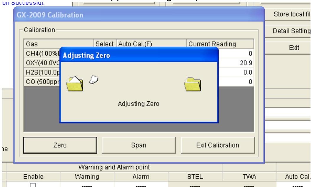
**Figure 24: Adjusting Zero Window**
