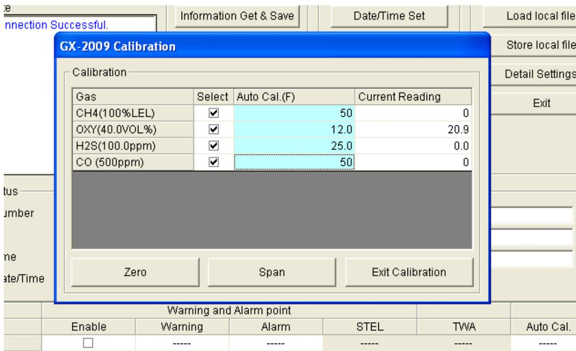
**Figure 23: GX-2009 Calibration Window**
