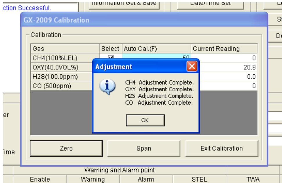
**Figure 25: Adjustment Complete Window, Zero**
