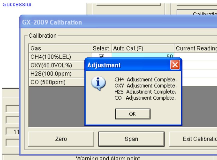
**Figure 29: Adjustment Complete Window, Span**
